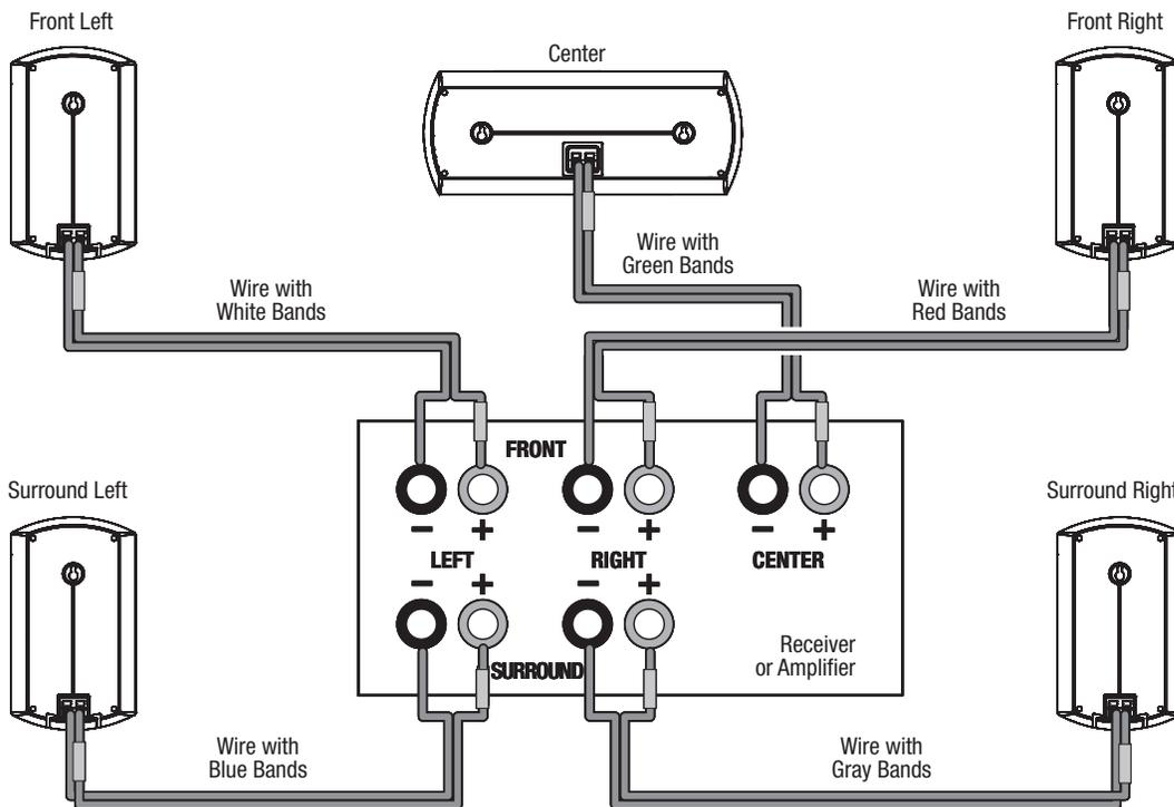
**IMPORTANT:** Make sure the (+) and (-) bare wires do not touch each other or the other terminal. Touching wires can cause a short circuit that can damage your receiver or amplifier.
